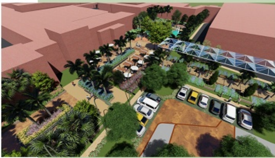
Green parking and bioswale replacing conventional drainage system.
