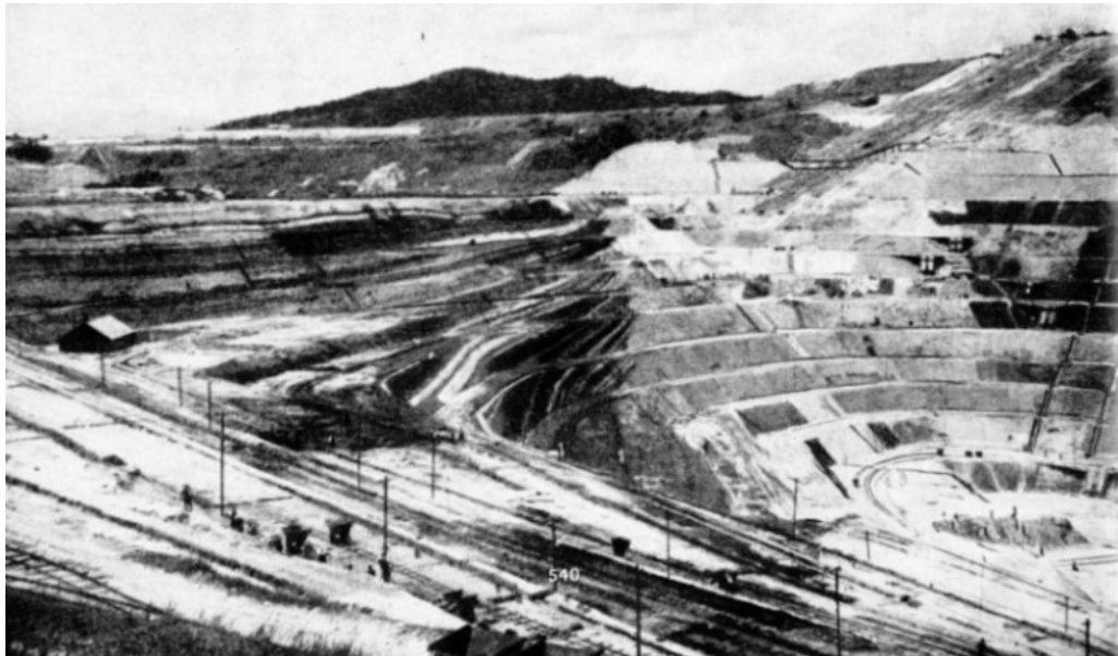
OPEN CAST MINE in the State of Selangor, Malaya. The mine is excavated in a series of benches along which rails are laid to convey the truckloads of excavated material to the inclines which lead to the surface, where the tin-bearing ore is extracted and treated.
