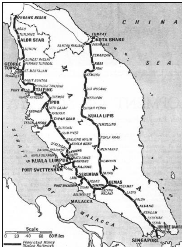
A SCALE MAP of the routes operated by the Federated Malay States Railways. There are 946 miles of metre gauge track open, and also 121 miles of metre-gauge track leased to the system.
