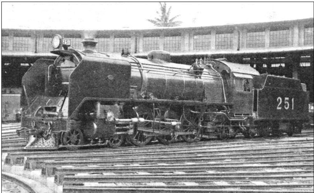
ONE OF THE LATEST TYPE of "Pacific" locomotives employed on the Federated Malay States Railways' system. Express trains in British Malaya are hauled chiefly by two- or three-cylinder 4-6-2 engines.
